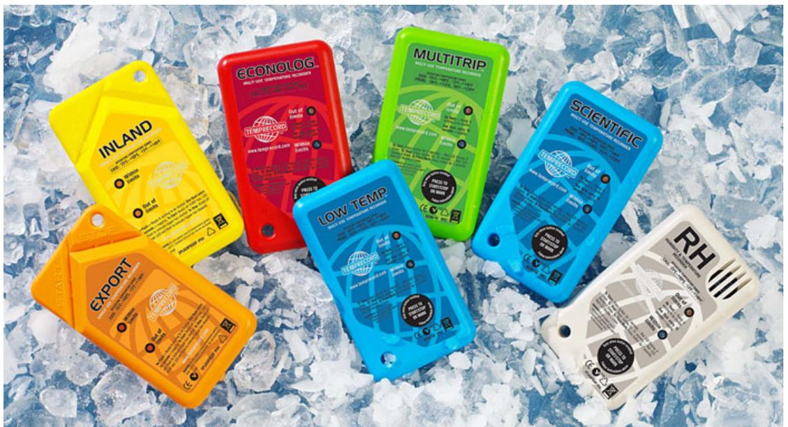
There are several variants of "Mk3" loggers. The Inland and Export models are single use loggers that are started and stopped by snapping off corner tabs. The remainder of the Mk3 loggers are multi-use loggers. The Scientific and RH (relative humidity) loggers are individually corrected and have enhanced accuracy specifications.
