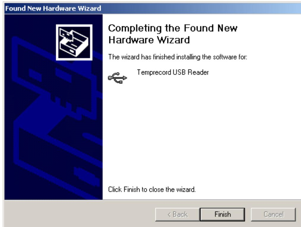
At this point, the whole process will repeat for the driver named "USB Serial Port". After this has completed (make the same selections as detailed above for installation of the Temprecord USB Reader) your reader should be ready for use. If you encounter difficulties, you can try to [install the USB drivers manually](#)
