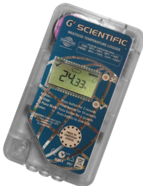
The G4 logger is a completely new design that incorporates a Liquid Crystal Display (LCD). As well as providing the logging functions of the Mk3 loggers, the G4 logger displays the most recent logged temperature. It can also display the temperature on demand, and various statistics computed from the logged data.
