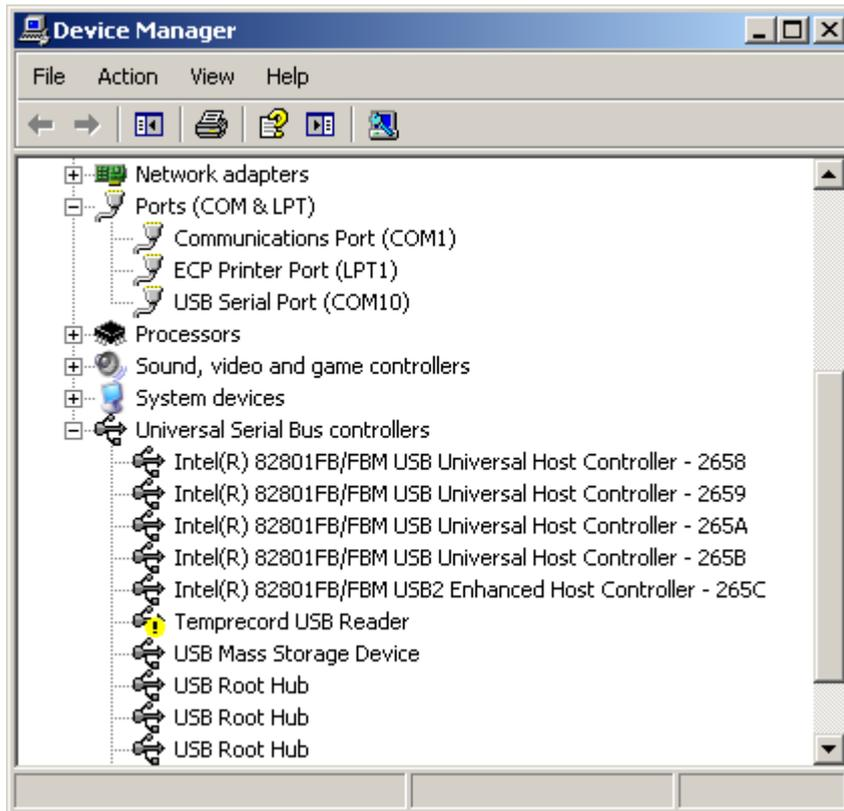
If the driver for the Temprecord Reader Interface is missing or incorrectly installed, and the a yellow exclamation mark will show beside the USB symbol in the hardware list. Right-click the **Temprecord USB Reader** entry and select **Update Driver**. The following dialog will display:
