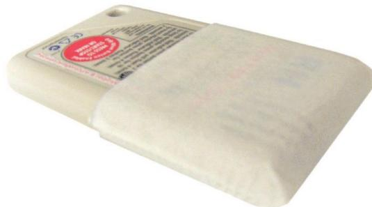
The dust covers have been designed and manufactured to allow maximum airflow to reach the humidity sensor while at the same time preventing dust and other airborne contaminants settling on or around the RH sensor. The dust cover slides over the logger and is held in place by the tight fit of the cover around the logger case.
