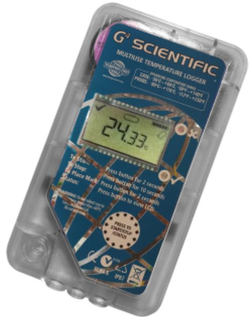
Under normal operation, pressing the button briefly moves between the various screens in the logger in a circular fashion, i.e. when the button is pressed while the last screen is displayed, the first screen (called the "home" screen) is displayed.
